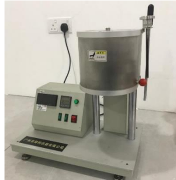
Melt flow indexer used for melt flow rate test (maximum 400°C)
