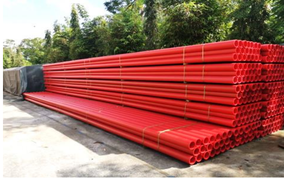
HDPE pipes finished products in piece form being stored at PPI prior to transportation to project site
