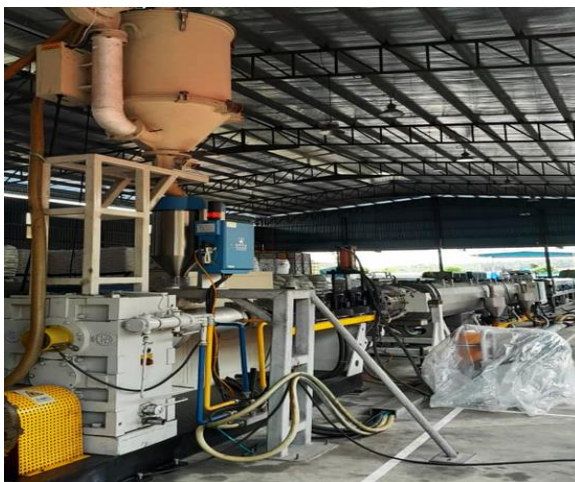
View of mixing tower of pipe extrusion line, dried raw materials (being HDPE resin and masterbatches) will be loaded
