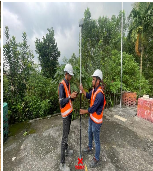
Tracing officers checking the coordinates using the boundary mark at site
