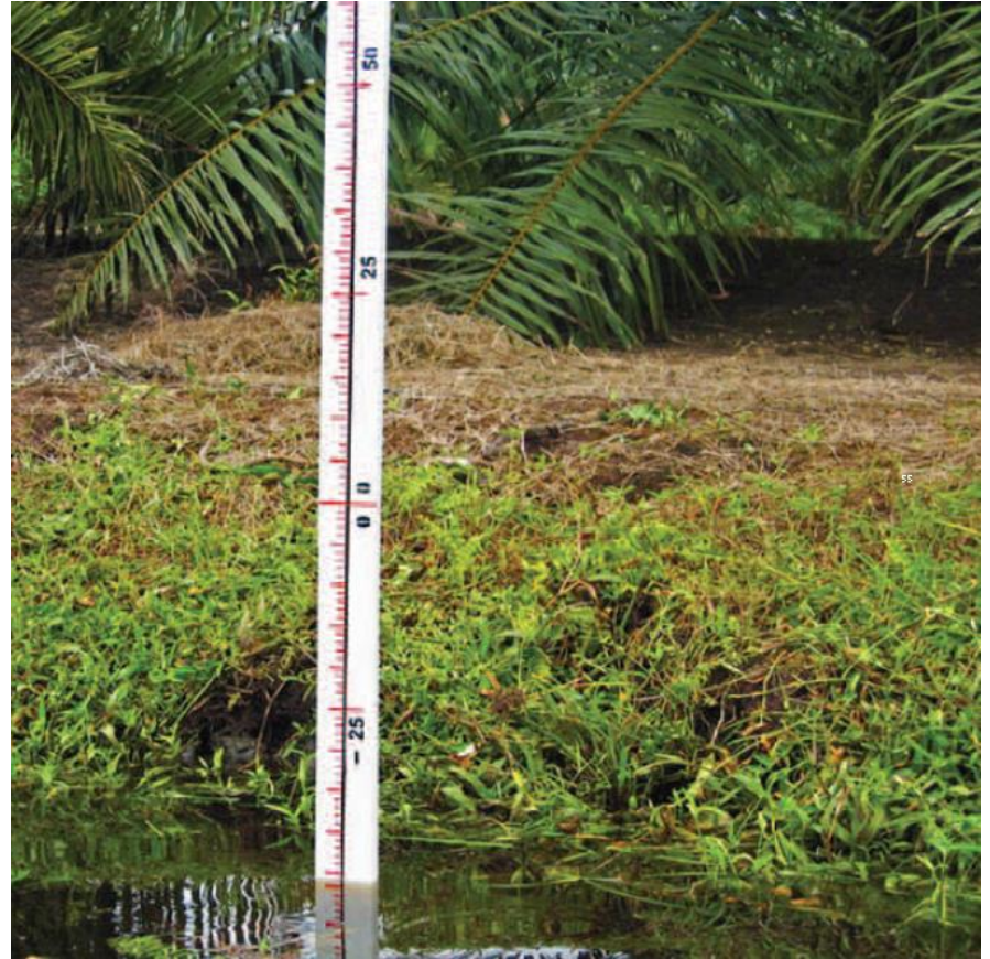
Water level monitoring point (optimally 50-70cm below the bank)
