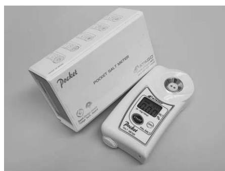
Digital pocket salt meter used for measuring the concentration of salt content in food products
