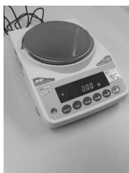
Electronic precision balance used for measuring ingredients in precise weight
