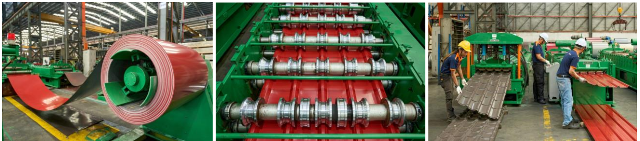
1 st picture: Medium to high tensile mild steel which is aluminium-zinc coated or colour coated is fed into the forming machine; 2 nd picture: A series of rollers to form a desired profile; 3 rd picture: The roofing sheet is then cut to the desired length.
