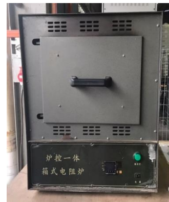
Muffle furnace used for ash content test (up to 1000°C)
