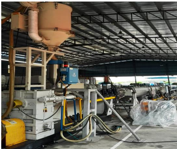
View of mixing tower of pipe extrusion line, dried raw materials (being HDPE resin and masterbatches) will be loaded
