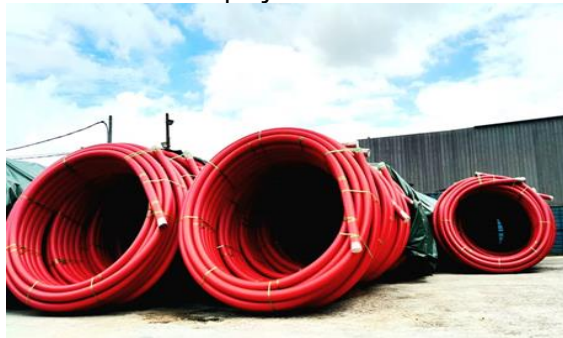
HDPE pipes finished products in coil form being stored at PPI prior to transportation to project site
