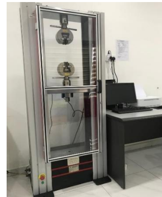
Tensile machine used for elongation at break, tensile strength and compression test (maximum 5,000 Newton)
